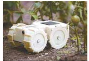
Equipped with a mini string trimmer, "Tertill" robot takes out newly emerged weeds in gardens. A sensor on front detects weed and activates trimmer, which is out of sight under body of robot.
