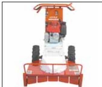
Walk-behind brush cutter has small plates on front that swing to keep rocks and debris from shooting out.
