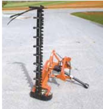
Hydraulic drive provides cutting action no matter what angle the bar is at, from horizontal to vertical.
