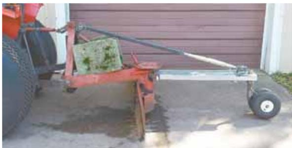
A 2-wheeled, triangle-shaped attachment makes Timothy Hoopman's 3-pt. mounted blade work more like a road grader.
