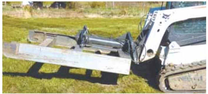
He can tilt the blade up and down and left or right, thanks to a unique mount that uses an old sheep's foot roller tongue and bushings.
