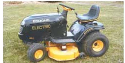
Brian Edmond converted this gas-powered lawn tractor to electric. It has 3 motors: one for the drive system, and 2 smaller ones mounted directly to the mower blades.
