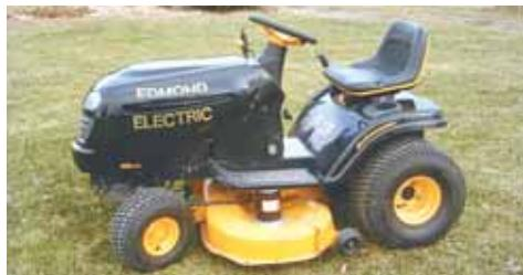
**Brian Edmond converted this gas-powered lawn tractor to electric. It has 3 motors: one for the drive system, and 2 smaller ones mounted directly to the mower blades.**
