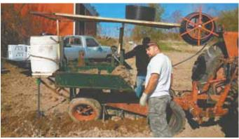
Stewart Holliday uses this modified 1-row tree planter to plant asparagus. It prepares the trench and makes it easy to drop the crowns in, and it also buries drip tube irrigation beneath the crowns.
