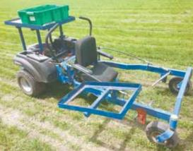
Holliday converted a Dixon zero-turn riding mower into this asparagus harvester, eliminating the need to bend to pick spears.
