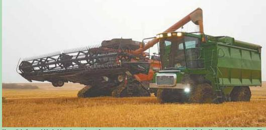
Shane Schafers and his dad bought an airport foam pumper and turned it into this one-of-a-kind, self-propelled grain cart. They built a 900-bu. grain box and replaced the original cab with one from a Case 2380 combine
