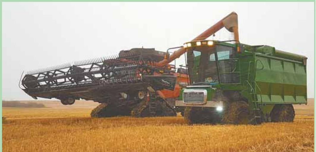
Shane Schafers and his dad bought an airport foam pumper and turned it into this one-of-a-kind, self-propelled grain cart. They built a 900-bu. grain box and replaced the original cab with one from a Case 2380 combine.
