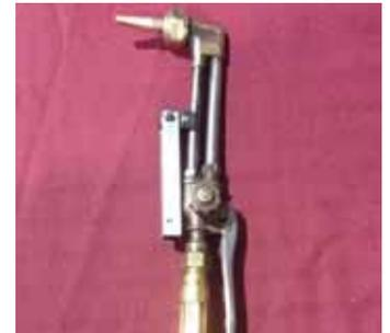
To light torch you fold striker all the way up and pull on the trigger. Unit folds out of the way when you’re done using it.
