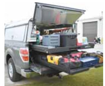
“SlideZilla” sliding tool trays can be stacked 2-high, with one between the wheel wells and one above.
