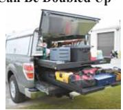
"SlideZilla" sliding tool trays can be stacked 2-high, with one between the wheel wells and one above.
