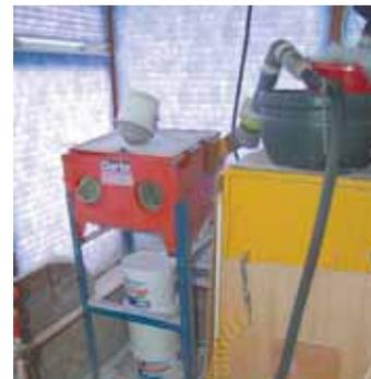
**Andrew Sewell hooked up a shop vac to his “glassblasting cabinet” to turn it from positive to negative pressure and stop it from leaking (above). A homemade bleed valve is used to regulate vacuum in the chamber.**
