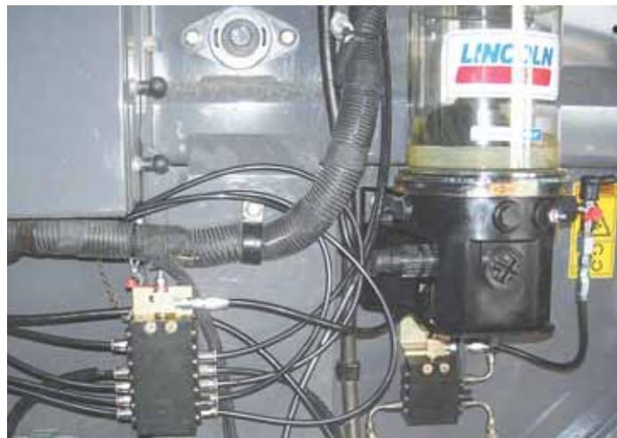
**Lincoln auto-lube system installed on a Gleaner combine.**
