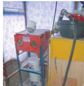
**Andrew Sewell hooked up a shop vac to his “glassblasting cabinet” to turn it from positive to negative pressure and stop it from leaking (above). A homemade bleed valve is used to regulate vacuum in the chamber.**
