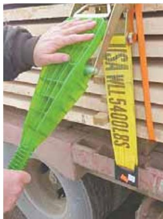
**Jaw at top of tool slips over bottom of ratchet handle, providing extra leverage to properly tension ratchet straps.**
