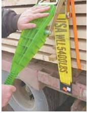
Jaw at top of tool slips over bottom of ratchet handle, providing extra leverage to properly tension ratchet straps.
