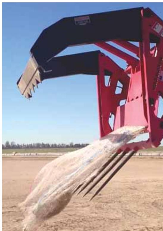
Loader-mounted round bale splitter holds onto net wrap so you can release it in a convenient location and keep it out of your feed grinder.
