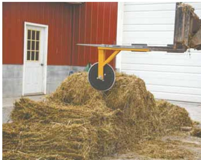
Sharpened coultter mounted on a tubular steel arm slides over skid loader fork. Down pressure alone is enough to slice through bales.
