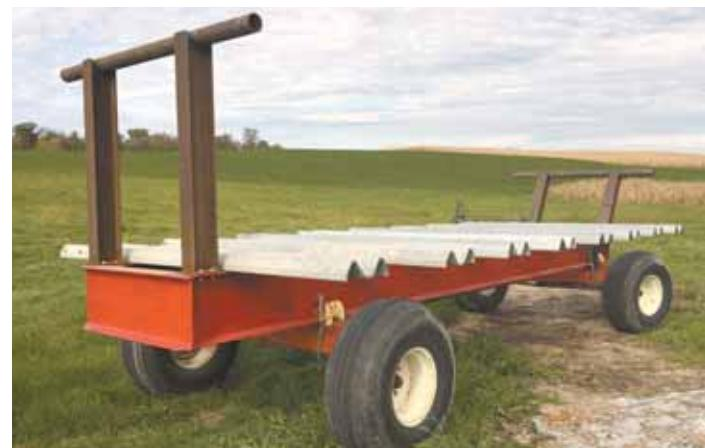
**Heavy duty bale wagon is built sturdy enough to support 27 big round or square bales without twisting or bending.**
