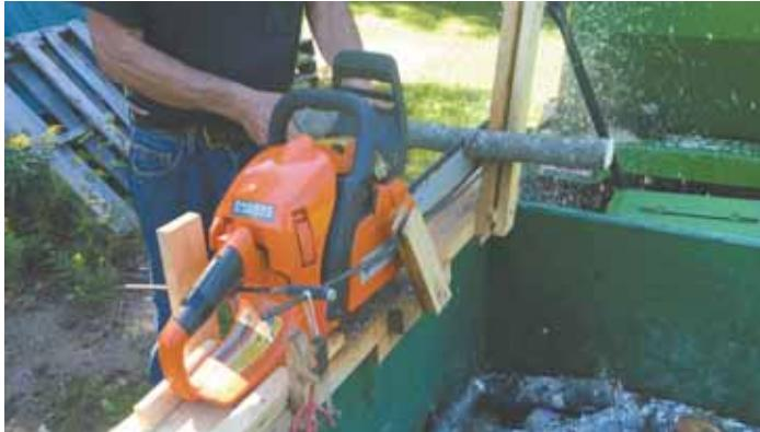
**Wooden chainsaw holder is fitted with brackets that fit onto side of yard trailer. As Clark pushes tree limbs down on top of chainsaw bar, the cut piece falls into trailer.**
