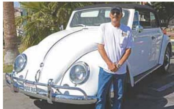
This Volkswagen Bug built by Richard Tupper is 40 percent larger than the real thing. It’s built on the chassis of a Dodge Ram pickup.
