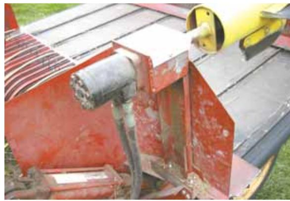
Paddle reel is mounted over throat of inverter at end of conveyor. A variable speed hydraulic control on tractor is used to adjust paddle speed.
