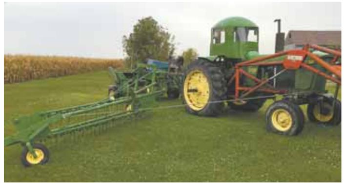
Home-built ditch rake brings mowed ditch hay into a windrow on side of road for baling. It'll handle a 10-ft. swath.
