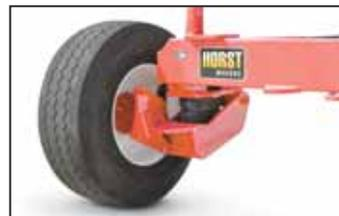
Shock absorber blocks mount on steel cases that float on pivot pins, allowing each wheel to respond independently.
