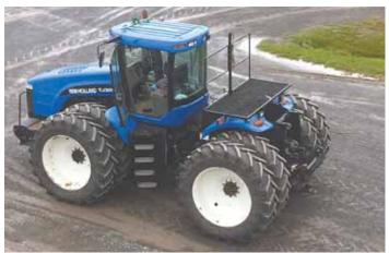
Max Kaiser made a secure platform for pruning trees along field edges by mounting a home-built metal deck on back of his New Holland 4-WD articulated tractor.
