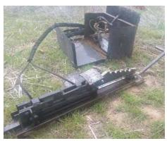
Terry Jacob uses his hydraulic culvert "reshaper" to fix damaged culvert ends that often plug up with heavy rains.
