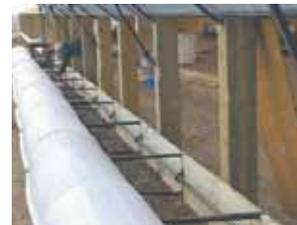
**Photo shows sidewall open and bunk tipped upside down for cleaning.**
