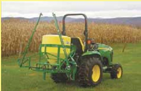
Alvin Wittmer's 3-pt. mounted sprayer comes with a 12 or 18-ft. boom that can be extended in 18 or 36-in. increments, and with an 80 or 35-gal. tank.
