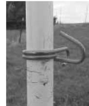
**Electric fence post has a 5-in. long steel spike at the bottom that can be quickly pushed into the ground. The electric wire is held on with a steel clip that slides over the post.**
