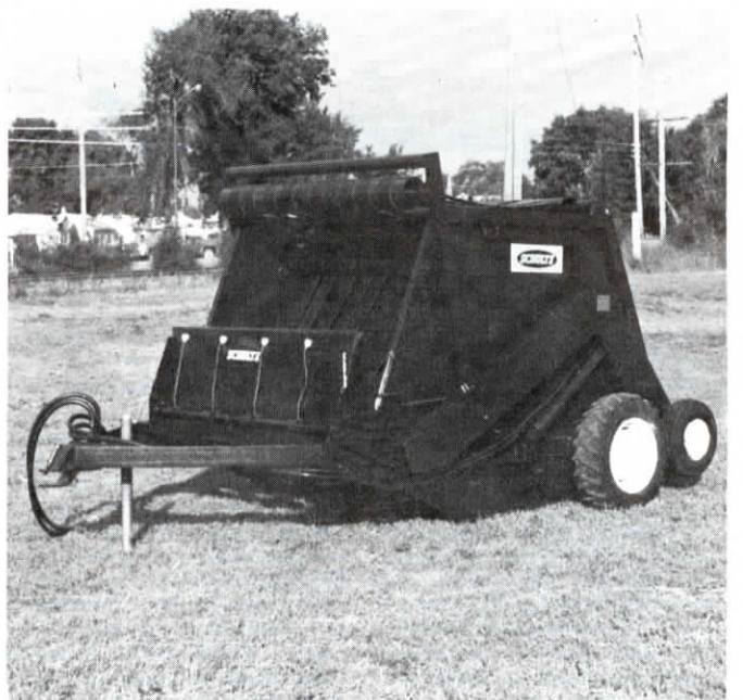
Nine belts (one-third less than most other belt-type balers) in the Schulz ground-driven baler form 5 by 5 ft. bales weighing approximately 1,500 lbs.
