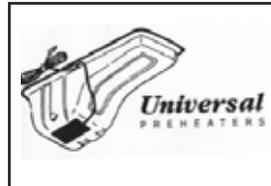
water tanks and even bulk oil tanks. The Preheater plugs into any 120 or 240 volt outlet and consists of a thin silicone fiberglass pad containing a metal grid. To install it, you clean an area on the bottom or side of the oil pan and press the pad onto it, then use silicone to seal the edges of the pad and place a flexible ceramic insulation pad over it. It is available in several models depending on the lube capacity. A 50 watt unit sells for \$44 and a 350 watt unit sells for \$133.
