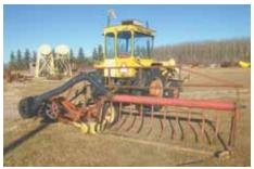
To keep the cutterbar clean on his New Holland mower, Dale Rogers modified the air reel from an old combine and then added a blower off a Gleaner sidehill combine.
