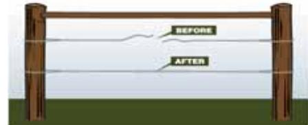
Wrapping the **TwistSplice** around a broken wire, or the **TwistEnd** to a terminating wire at an end post, creates a solid, rod-like connection.
