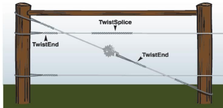
**TwistEnds** create a secure loop around a post or a radius around a corner post. **TwistSplices** are said to be stronger than the original wire's breaking strength.
