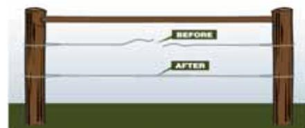
Wrapping the TwistSplice around a broken wire, or the TwistEnd to a terminating wire at an end post, creates a solid, rod-like connection.
