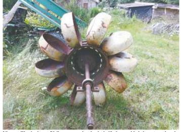
Vincent Theriault cut 20-lb. propane bottles in half, then welded them to a tire rim mounted on an axle to create this water wheel. He mounts it at the end of a culvert, connected to an alternator that charges batteries.
