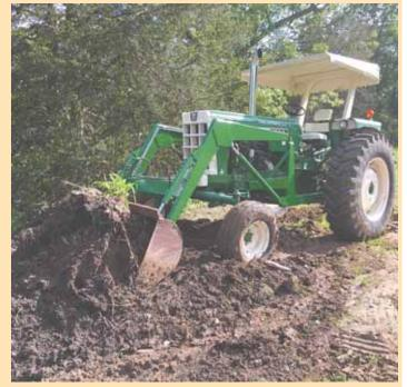
When the gas engine on his Oliver 1650 started to fail, Andy Buelow replaced it with a Cummins diesel as well as a 3-speed hydroshift from an Oliver 1855. He also added a front-end loader.
