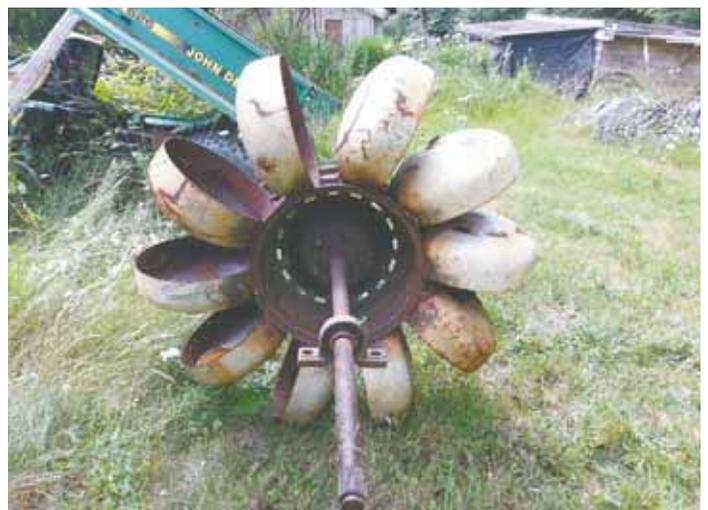
Vincent Theriault cut 20-lb. propane bottles in half, then welded them to a tire rim mounted on an axle to create this water wheel. He mounts it at the end of a culvert, connected to an alternator that charges batteries.
