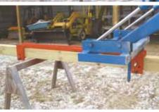
Post is first placed on a pair of sawhorses. Lamb lowers post handler down until both saddles straddle post. Then he inserts steel pins through saddles and tightens threaded rods into side of post to keep it from sliding when he lifts it up.
