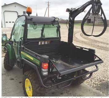
UTV-Mounted Rock Hawk is designed to pick up rocks in the field and then swing them over into a steel replacement box.
