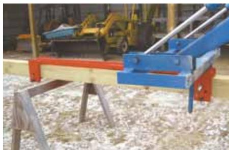
Post is first placed on a pair of sawhorses. Lamb lowers post handler down until both saddles straddle post. Then he inserts steel pins through saddles and tightens threaded rods into side of post to keep it from sliding when he lifts it up.
