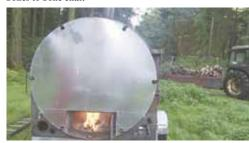
There is a firebox underneath the 8-ft. combustion chamber. No external power source is needed.
