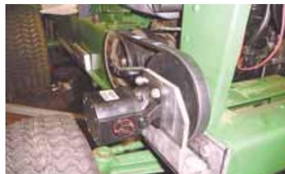
Dennis Gintowt built this front-end loader for his 1972 Deere 112 garden tractor. With weights on back of tractor he can pick up as much as 500 lbs. Hydraulic pump is self-driven off the engine and positioned so it doesn’t hit tractor’s front wheel.
