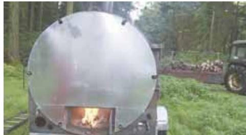
There is a firebox underneath the 8-ft. combustion chamber. No external power source is needed.
