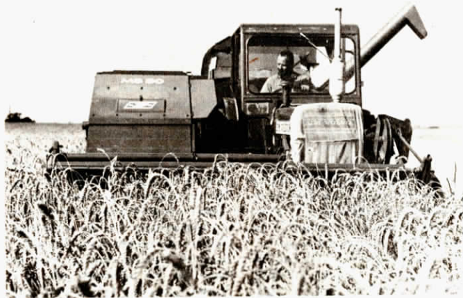
Combine mounts on most tractors in 40 to 60 hp range and comes with 10 ft. wide header.
