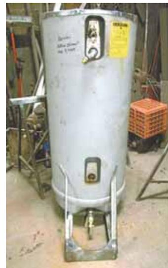
He attached a garden hose fitting at top of heater to provide an overflow and installed a gravity float valve in drain hole fitting at the bottom.
