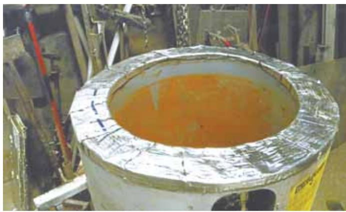
Gene Boehler cut the top off a 50-gal. water heater and installed an electric sinker-type tank heater, converting the unit into an insulated livestock waterer.
