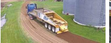
Spreader replaces belly dump trailer's existing push block with an air-operated, 16-in. high steel blade just under 8 ft. wide.
