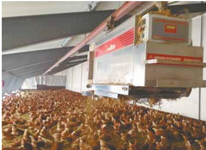
Robotic spreader from JH Agro spreads straw, sand and other bedding material with no need for a shovel or fork. Battery-powered unit moves back and forth on rails.
