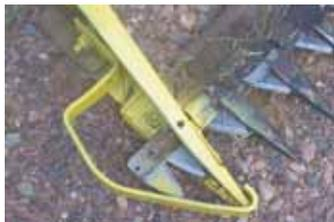
Metal guide pushes uncut grass away from end of knife on Jaster’s Deere 7-ft. pull-type sicklebar mower so that it won’t plug up. Guide also protects knife from rocks.
