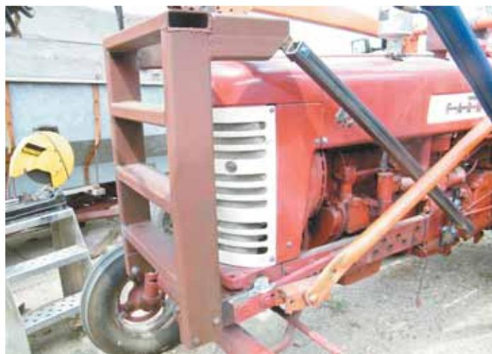
Heavy-built guard protects the front end on Swensen’s IH 450 loader tractor.
