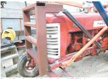
Heavy-built guard protects the front end on Swensen's IH 450 loader tractor.
