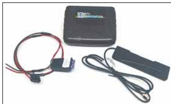
**New "hotspot" device connects through Verizon or AT&T to provide WiFi in moving vehicles or farm equipment.**
