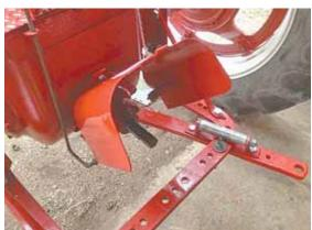
Pto guard is hinged to make it easier to connect pto shaft.
