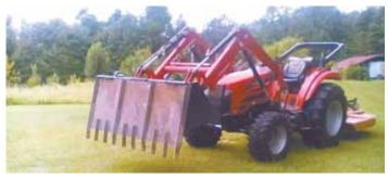
Blade is sized to match a standard 6-ft. bucket and drops about an inch below bucket's cutting edge. Teeth extend about 4 in. below edge of blade.
