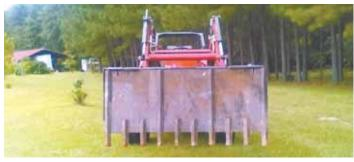
Bucket-mounted dirt blade lets Ledbetter blade dirt without getting dirt in bucket. It can be quickly popped off so bucket can be used to lift and load material.
