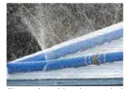
Giant perforated hose is pressurized by a gas-powered pump to help protect properties from fire. It can drench an area with more than 25,000 gal. per hr.
