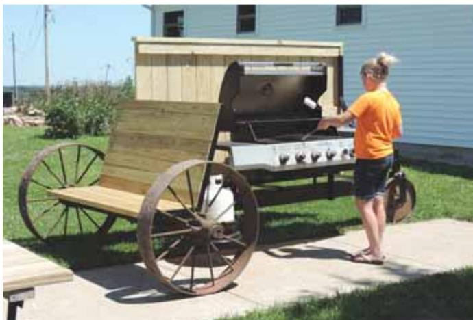
Barbeque gas grill mounts on a big 3-wheeled metal stand that also supports a wooden bench and a 5 1/2-ft. high wooden windbreak, which shelters the cook.
