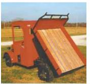
Robert Sallee converted a Cub Cadet riding mower to look like an International Harvester truck from the 1930's. It's equipped with a 4 by 5-ft. dump box with a wood bed.
