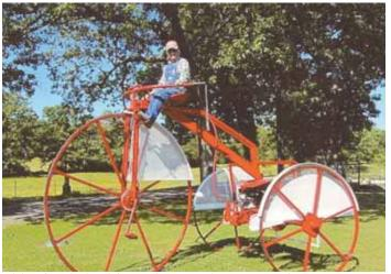
William Green's giant 9-ft. tall, high-wheel tricycle can carry 2 adult passengers on back. Rear wheels are driven by a 3 1/2 hp. engine that belt-drives the hydrostatic transmission off an old riding mower.
