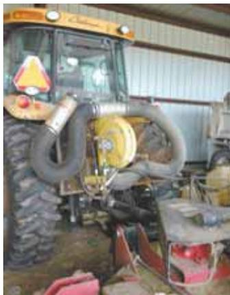
Terry Jacob keeps his big mower decks clean with this hydraulic-operated fan and 6-in. hose mounted on back of his tractor.
