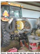
clean with this hydraulic-operated fan and 6-in. hose mounted on back of his tractor.
