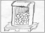
Large opening cut into 275-gal. fuel oil tank is used to store firewood. Cut-off piece serves as a protective awning.
