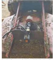
Photo at left shows mounting plate added to back of mower deck. At right, hydraulicpowered driveshaft powers pto drive.
