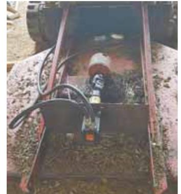
Photo at left shows mounting plate added to back of mower deck. At right, hydraulic-powered driveshaft powers pto drive.
