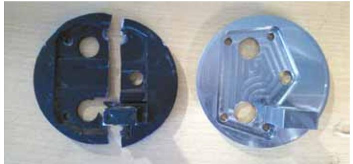
Replacement hydraulic control valve plate for Case IH tractors (right) is machined from 4-in. solid steel.
