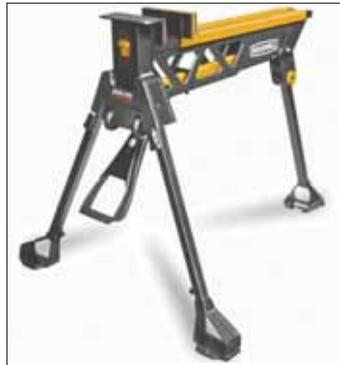
get your projects up off the ground to a comfortable working height. The vise is closed by pumping a foot pedal, freeing both hands for positioning and clamping. It's made of solid steel and, according to the company, it has 10 times the clamping power of a regular vise.
