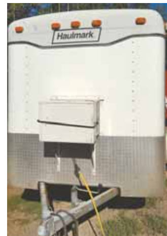
Raindrop Farms needed more storage for their fresh flower business, so they converted an 8 by 10-ft. cargo trailer into a mobile cooler that makes use of a window-style air conditioner controlled by a "Cool Bot".
