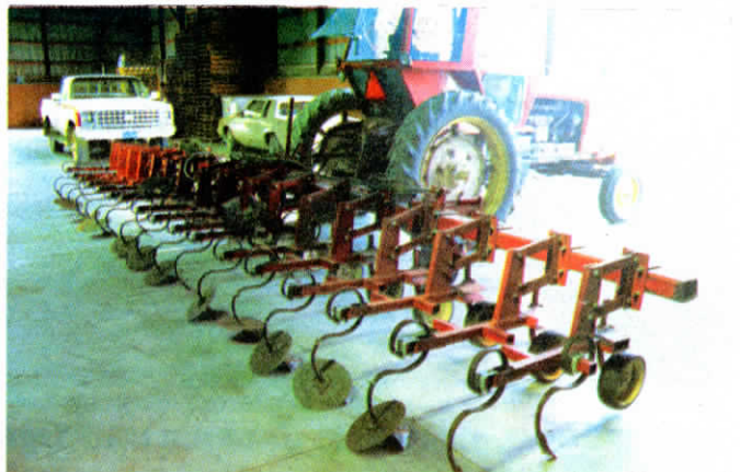
Ricke removed two shanks per row from 12-row, 30-in. Danish tine cultivator and turned it into 16-row, 20-in. cultivator. Disc opener over each shank breaks up slabs.
