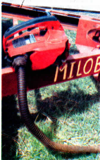
Buchholz removed saw's bar and chain and modified the exhaust pipe so he could attach flexible metal pipe.
