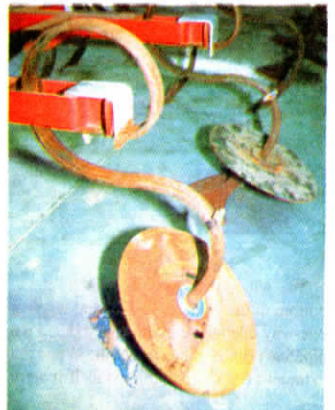
The 10-in. dia. disc opener is slipped onto each shank with washer above and below the disc.
