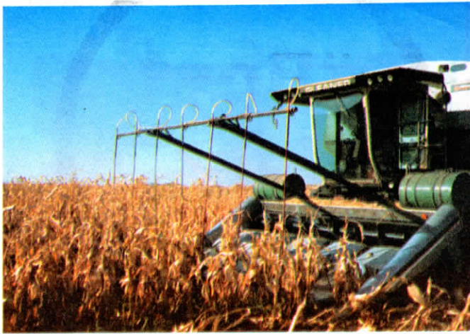
Fiedler mounted "drop tube" spraying system on header of his Gleaner combine.
